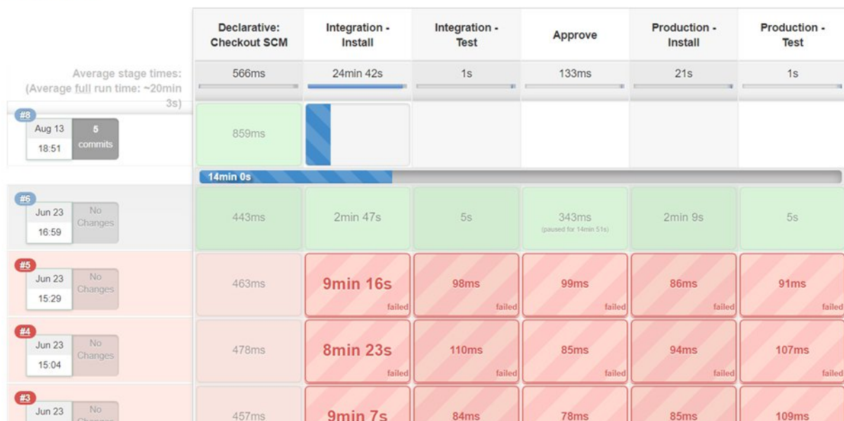
Figure 6: Jenkins pipeline with six stages for Zammad.
