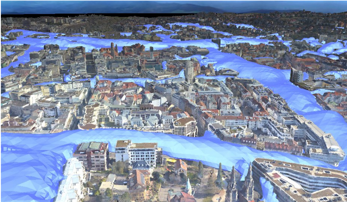
Figure 86. Screenshot of the interactive visualization. Iso surface for NO x are shown along with a city model (Stuttgart building scans).
